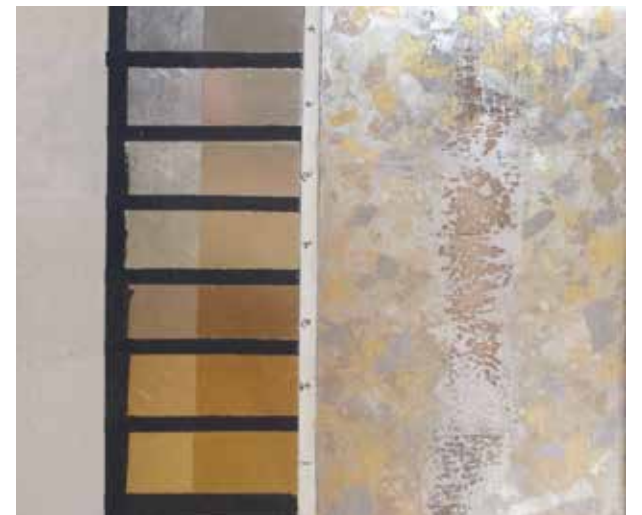
The gold-leaf wall on the Amels Aurora Borealis is protected with a lacquer finish.
